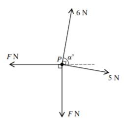
A particle P is in equilibrium on a smooth horizontal table under the action of four horizontal forces of magnitudes 6 N, 5 N, F N and F N acting in the directions shown. Find the values of  $\alpha$  and F. [6]
