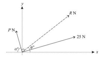
Forces of magnitudes P N and 25 N act at right angles to each other. The resultant of the two forces has magnitude R N and makes an angle of  $\theta^{\circ}$  with the x-axis (see diagram). The force of magnitude P N has components -2.8 N and 9.6 N in the x-direction and the y-direction respectively, and makes an angle of  $\alpha^{\circ}$  with the negative x-axis.
