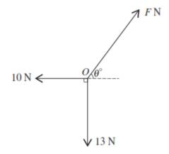
Three horizontal forces of magnitudes F N, 13 N and 10 N act at a fixed point O and are in equilibrium. The directions of the forces are as shown in the diagram. Find, in either order, the value of  $\theta$  and the value of F.
