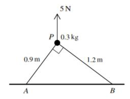
A particle P of mass 0.3 kg is held in equilibrium above a horizontal plane by a force of magnitude 5 N, acting vertically upwards. The particle is attached to two strings PA and PB of lengths 0.9 m and 1.2 m respectively. The points A and B lie on the plane and angle  $APB = 90^{\circ}$  (see diagram). Find the tension in each of the strings.
