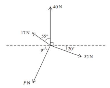
Coplanar forces of magnitudes 40 N, 32 N, P N and 17 N act at a point in the directions shown in the diagram. The system is in equilibrium. Find the values of P and  $\theta$ . [6]
