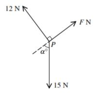
Three coplanar forces of magnitudes F N, 12 N and 15 N are in equilibrium acting at a point P in the directions shown in the diagram. Find  $\alpha$  and F. [4]
