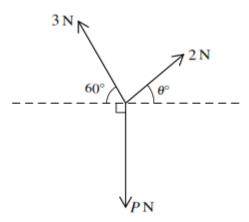
The three coplanar forces shown in the diagram have magnitudes 3 N, 2 N and P N. Given that the three forces are in equilibrium, find the values of  $\theta$  and P. [4]
