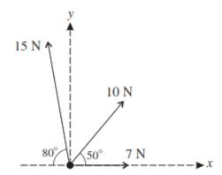
Forces of magnitudes 7 N, 10 N and 15 N act on a particle in the directions shown in the diagram.
