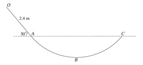
OABC is a vertical cross-section of a smooth surface. The straight part OA has length 2.4 m and makes an angle of 50° with the horizontal. A and C are at the same horizontal level and B is the lowest point of the cross-section (see diagram). A particle P of mass 0.8 kg is released from rest at O and moves on the surface. P remains in contact with the surface until it leaves the surface at C. Find
